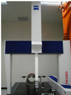
**Zeiss Coordinate Measuring Machine**
