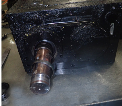
A Setco spindle that ran for years and eventually failed.
